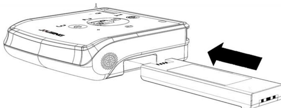
Figure 3 Installing the battery schematic
