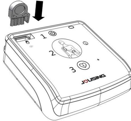
Figure 4 Pads Connector Insertion
