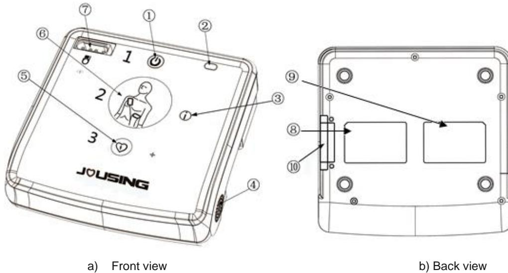
Figure 2 Controls and indicators on the iAED-S1
