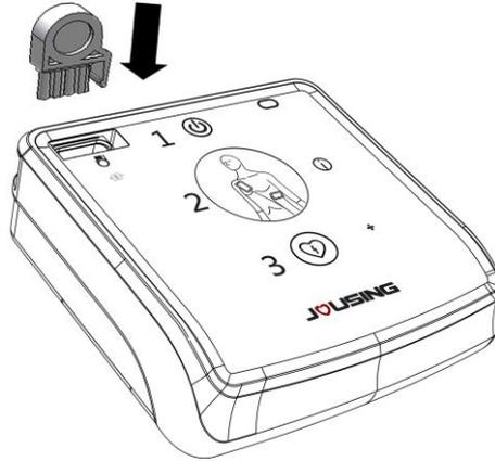
Figure 4 Pads Connector Insertion
